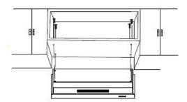
Step 3: Tighten the appliance with the 4 screws provided (M5\*26) to the four holes at the bottom of the cabinet
