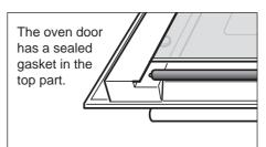
It is normal the opened gap between the top edge of the inner glass and the sealed gasket. This allows the cooling air circulation.
